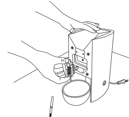
The cover plate is attached with magnets and can be easily removed by hand.
